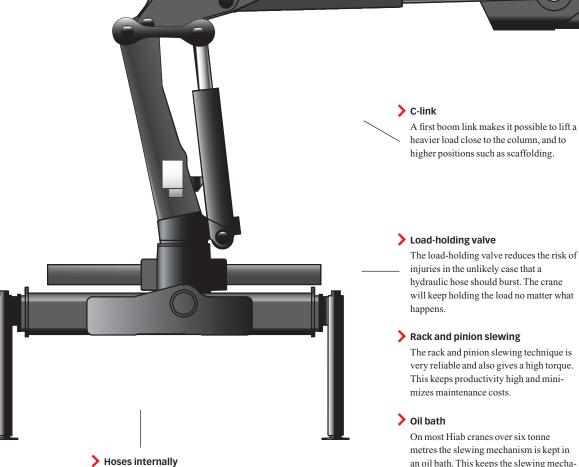
The hoses are run internally in the crane body and in the outrigger beam, where they are out of harm's way, thus reducing maintenance costs.
