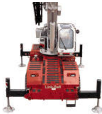
Intermediate Extended Outriggers 14' 8" (4.47 m) spread
