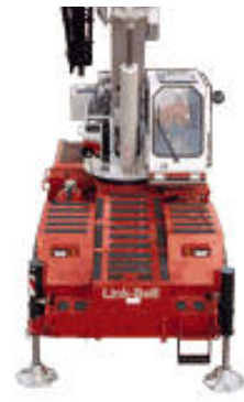
Fully Retracted Outriggers 8' 8-1/4" (2.64 m) spread
