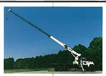
National Crane, America's truck-mounted hydraulic crane leader, features the industry's premier lineup of hard-working telescoping and articulating units. The medium-to-heavy-duty Series 500B telescoping crane (12½-ton capacity; 118-foot vertical reach) offers many advantages:
