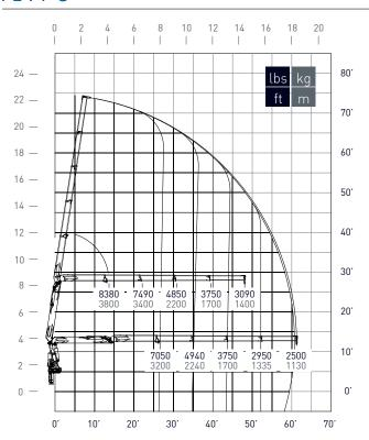
The stated performances can be obtained with 16° inclinated main boom.
