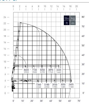
The stated performances can be obtained with 16° inclinated main boom.
