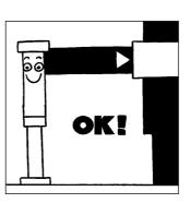
Level the crane so as it is always operated on a horizontal plane; check that the angle of inclination of the vehicle always does not exceeds five (5°) in any direction.
