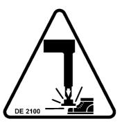
**DE 2100** Danger plate for crushing of lower limbs
