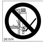
TIRANTI:NON SALDARE!FIXING ROD:DO NOT WELD!TIRANTS:NE PAS SOUDER!ZUGSCHRAUBEN:NICHT SCHWEISSEN
