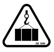
**DE 1686** Do not walk or stop under a suspended load
