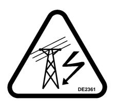
**DE 2361** Do not operate in proximity of electric high-tension lines
