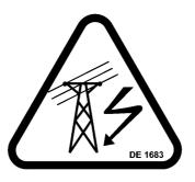
**DE 1683** Do not operate in proximity of electric high-tension lines
