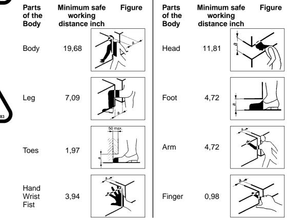
In conformity with "EN 349" Standard the minimum safe working distances to avoid crushing parts of the body.
