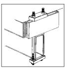
Check the tightening torque of the fixing rods of the crane. (fig. 20)
