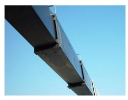
**Easy Glide boom wear pads** Easy Glide boom wear pads reduce the conditions that cause boom chatter and vibration. The net result is smoother crane operation.
