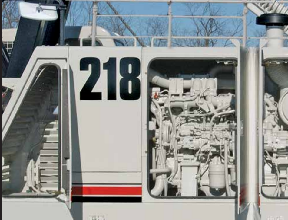
Excellent access for all routine engine and hydraulic maintenance
