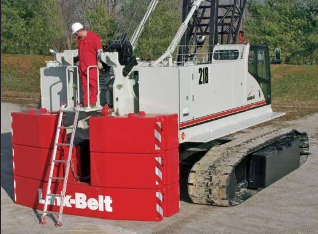
Counterweights lower completely to the ground
