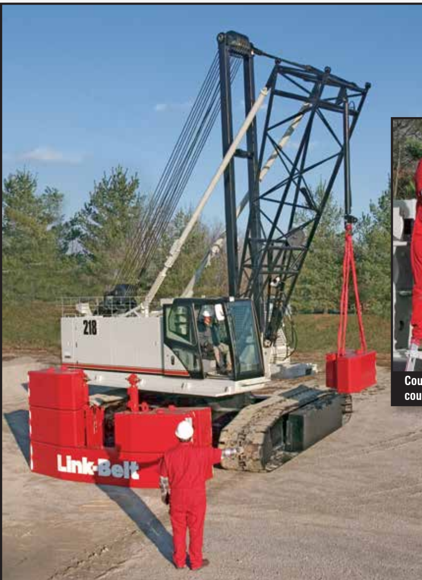
Counterweights lower completely to the ground
