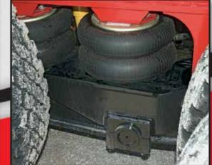
All **counterweight configurations** can be raised and lowered by hydraulic cylinders from the comfort of the operator's cab for ease of installation and removal.
