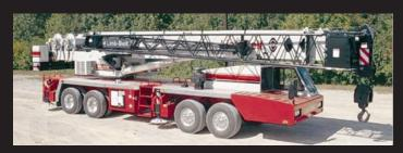
**Stowable Attachments** Swing-away lattice flys are easily stored for transportability or can be removed to meet specific road laws.
