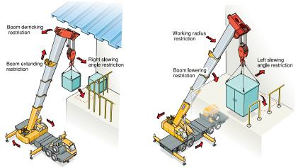
Slewing does not stop automatically, sound alarm only.
