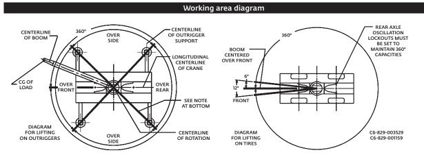
Bold lines determine the limiting position of any load for operation within working areas indicated.
