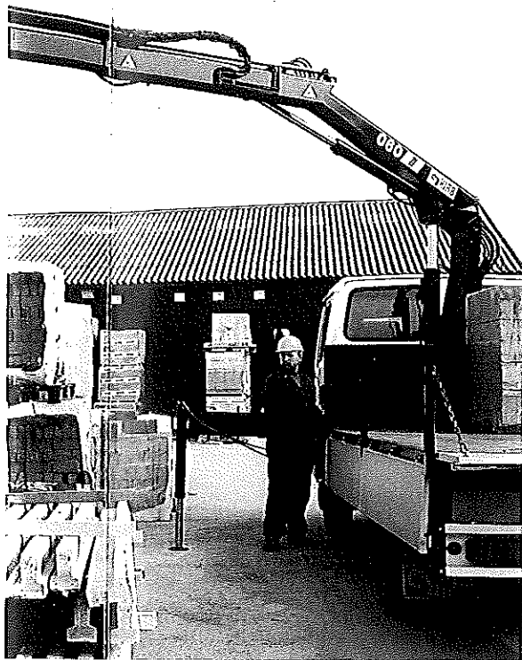
ile HIAB 060-2 with palletfork on a 7.5 GVW ton truck for inds of building materials.
