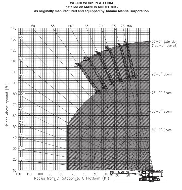
Limits of operation: Maximum load capacity = 750 lb
