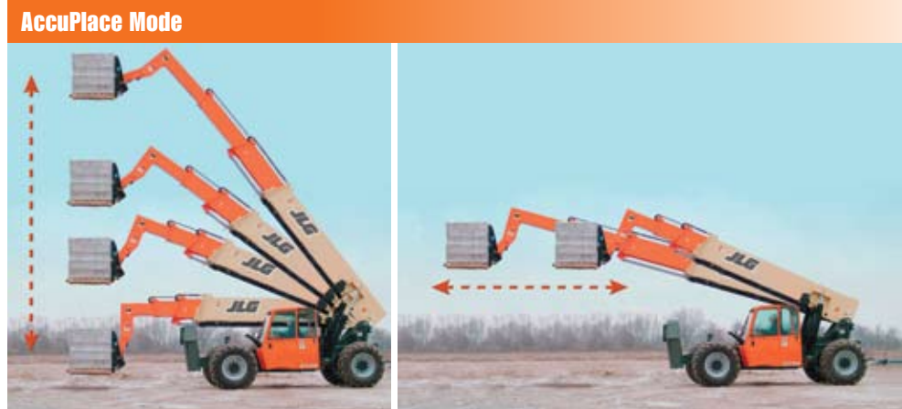
When AccuPlace is activated, the boom moves in a linear motion for more precise load placement—making work easier and faster for any trained operator.
