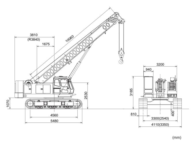
Note: The figures in parenthesis are in the case that crawler side frames are fully retracted.
