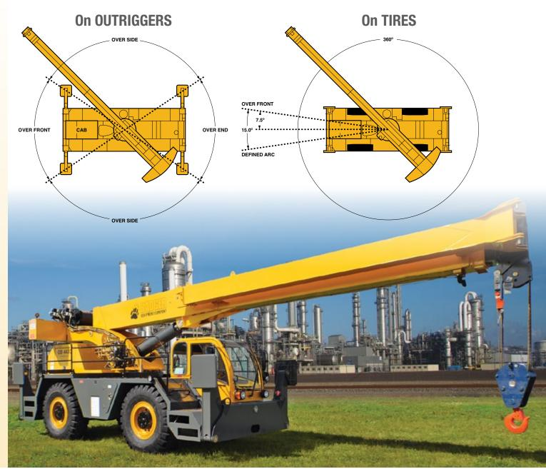
10. Pick and carry load ratings are shown in load chart for on tires. Boom must be above  $0^{\circ}$ .
