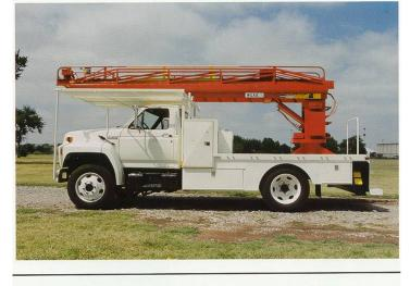
**MODEL 60 LADDER** ALL HYDRAULIC FIBERGLASS TOP SECTION
