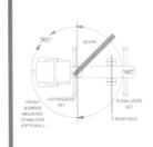
Front Mount crane operation is limited to 1800 outrigger to outrigger over rear, unless equipped w/optional front bumper mounted stabilizer. which permits full 360° area of operation.
