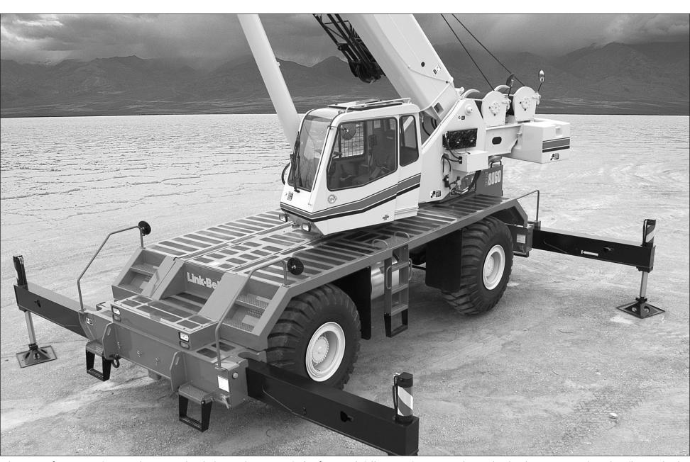
The RTC-8060 Series II features the new Link-Belt designed 38 to 115 ft. (11.6 to 35 m) full power, four-section boom that has boom wear pads with Teflon pucks that automatically lubricate the boom sections. As a result, no boom grease is required.
