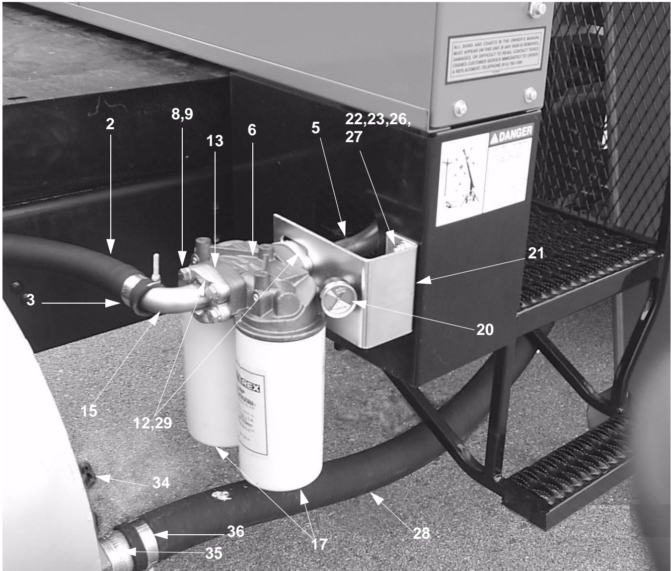
Hydraulic Reservoir & Filter Installation
