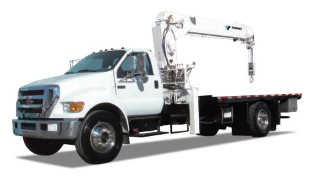
MAXIMUM LIFTING CAPACITY: 20,000 lbs EXTENDED LENGTH: 52.23'
