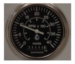
The EZ Reach 40 does not require its full engine power when moving. There are two basic settings for throttle control. The LOW throttle setting is approx. 1200rpm. The HIGH throttle setting is approx. 2000rpm
