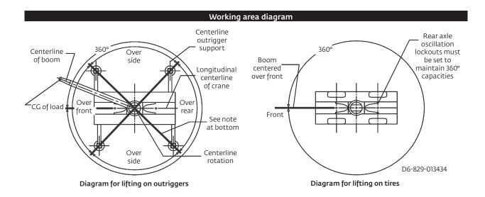
Bold lines determine the limiting position of any laod for operation withing working areas indicated.
