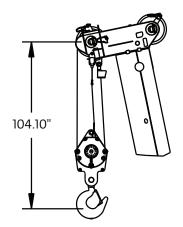
Dimensions are for largest Grove furnished hook block and headache ball, with anti-two block activated.
