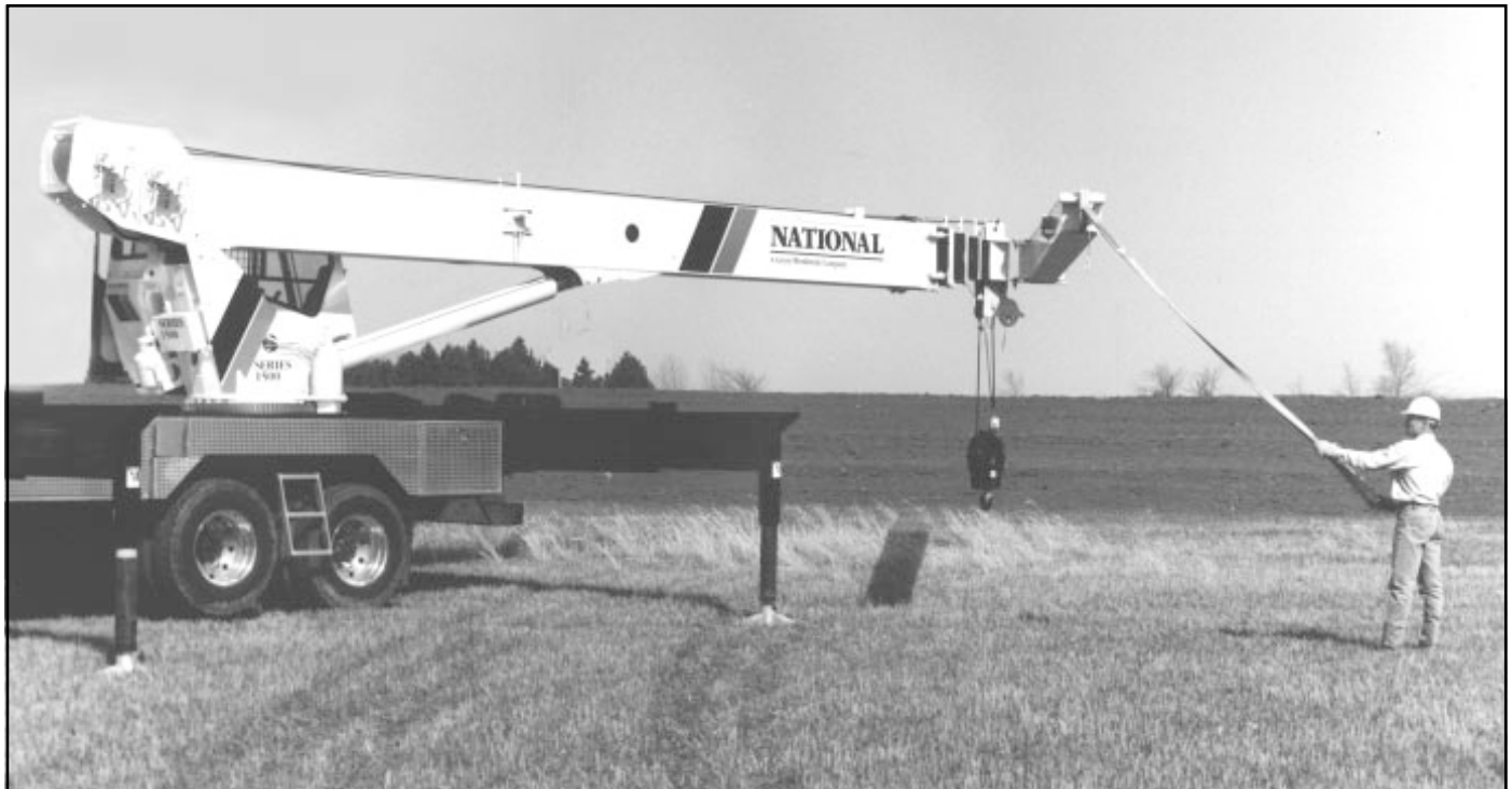
A National jib folds out into a working position quickly and easily.
