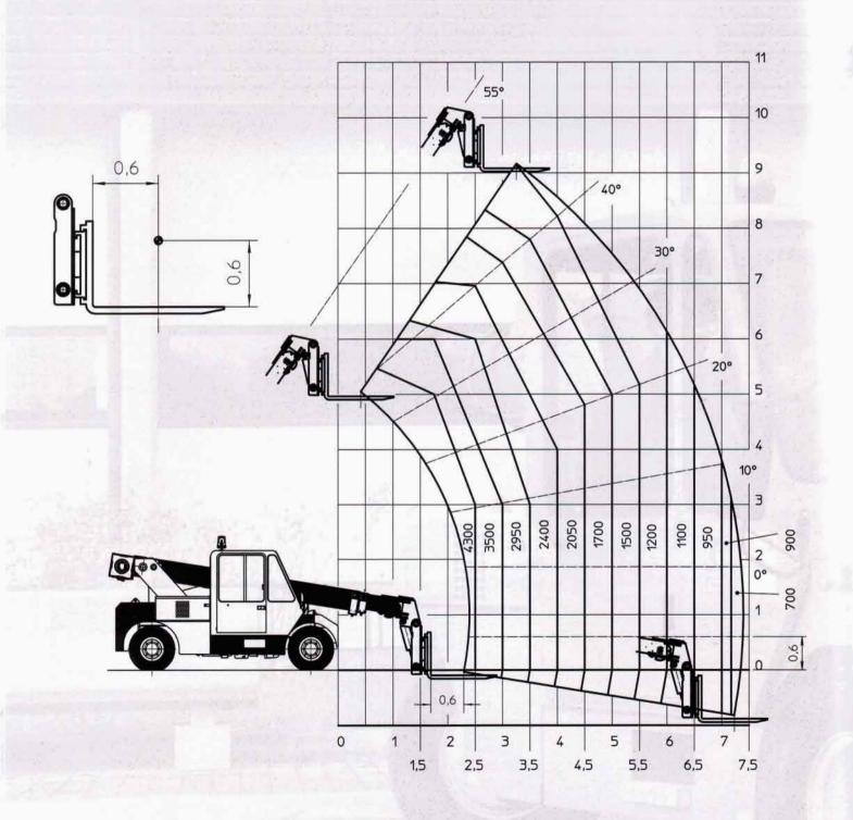
Lifting capacity chart (tonnes)
