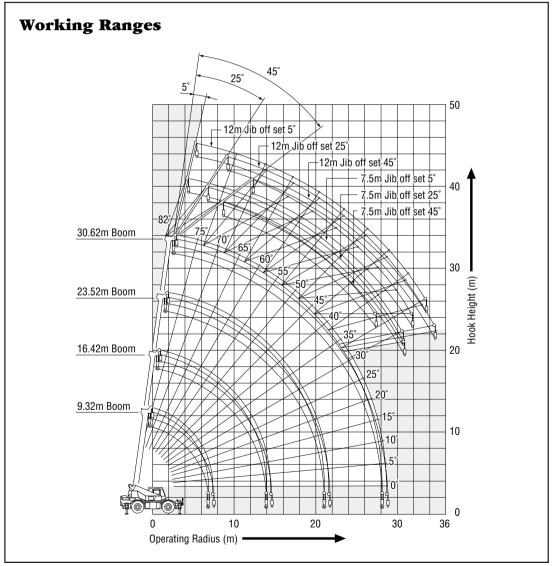
$^{\star}\mbox{Boom/jib}$  bending with load is not involved in figure of working ranges.
