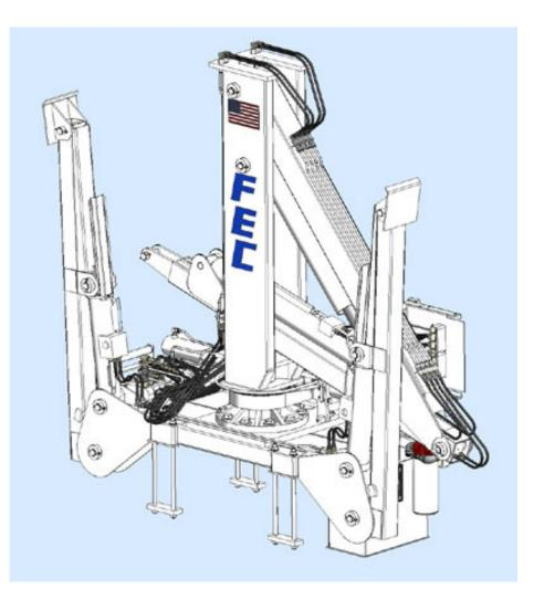
FEC's model 1815 tire service crane offers fold out style outriggers for extra stability. Rack/chain and pinion rotation system with superior durability. Load holding valves on all lift cylinders, chrome plated cylinder rods and walls. Heavy duty PTO and hydraulic pump.
