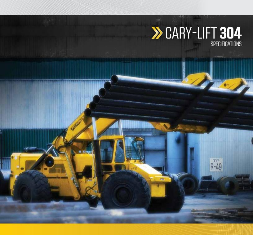
Ruggedly built to perform for the long haul, the Cary-Lift 304 offers a number of engineering advantages, including an overhead lift arm design that provides maximum visibility when lifting or moving loads. Featuring components like heavy-duty 4-wheel drive axles and a load-sensing hydraulic system, the 304 is stronger and smarter, allowing it to tackle the most demanding material handling jobs time and again.
